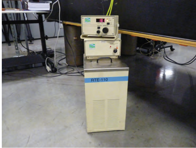
Figure 2.5: LED lighting cooling water chiller
